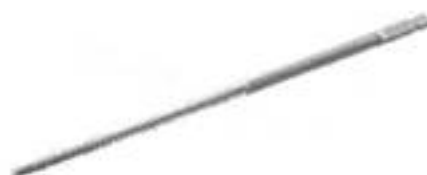
311.460 1 Tap for 4.5mm Cortex Screws total length 125mm, thread length 70mm predrilling: 3.2mm dia.
